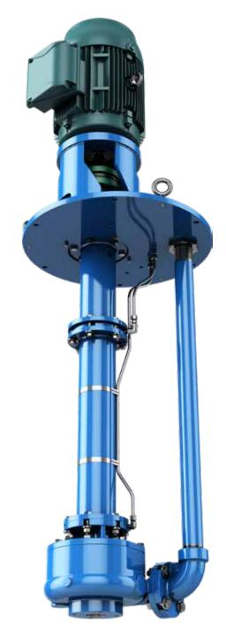
The CV 3171 is a recessed impeller, circular volute type sump pump. Ideal for large solids and shear sensitive fluids. It will pass any solid that will pass through the discharge pipe. Circular volute minimizes radial loads, making this the ideal pump for low flow process applications.
