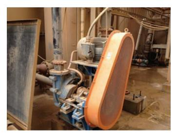
The 125XHD pump has surpassed 5,000 hours of operation with no issues beyond standard maintenance procedures on the packing.
