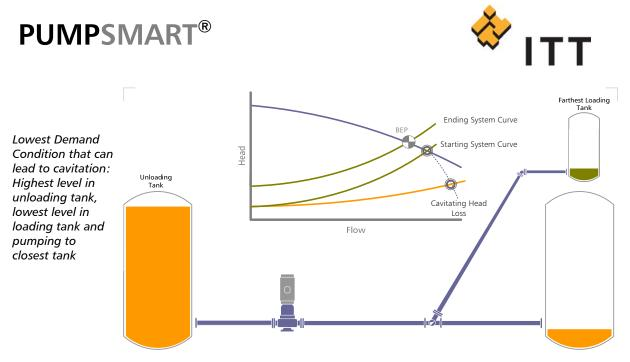
**Challenge #2 – Low suction tank level resulting in cavitation** – When tank unloading first starts, the liquid level in the tank being unloaded is sufficient to prevent the unloading pump from cavitating. As the level in the tank drops, the pump may begin to cavitate as suction pressure drops. Cavitation leads to reduced pump reliability and can also reduce product quality.
