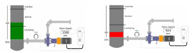
If cavitation is a concern for lower tank levels, pump speed and pump flow can be automatically reduced as the tank empties. In this example tank level is correlated to the suction gauge pressure.
