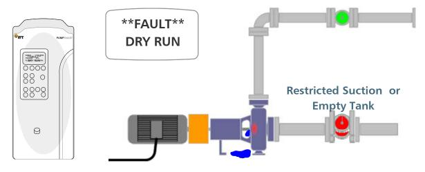
PumpSmart will detect a dry run condition and can be configured to automatically shut down the pump to avoid a catastrophic mechanical seal failure.
