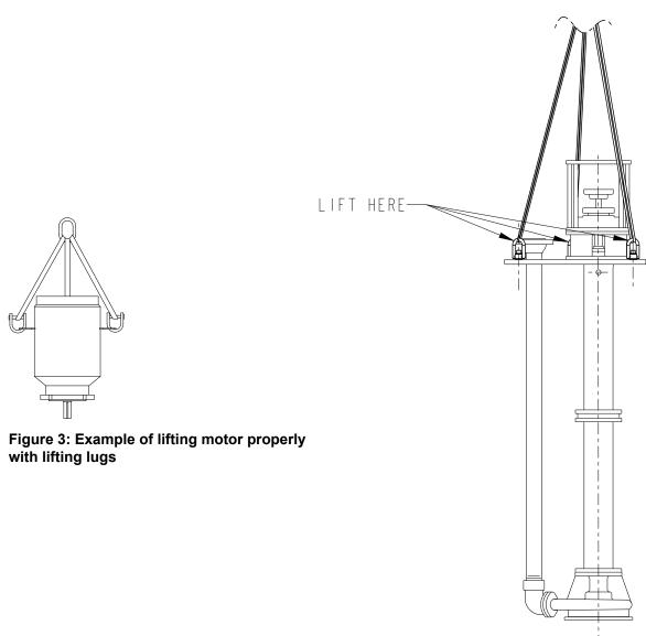
Figure 4: Example of lifting pump properly with sling
