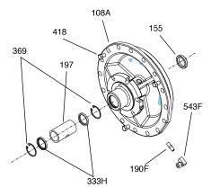
Figure 41: Steady bearing reassembly
