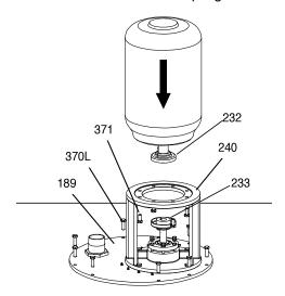
Figure 47: Motor and coupling reassembly
