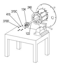
Figure 33: Bearing Shell and Shaft Removal
