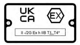
Figure 7: Typical UKCA Ex nameplate
