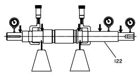
Figure 36: Shaft inspection
