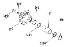
Figure 40: Steady bearing housing
