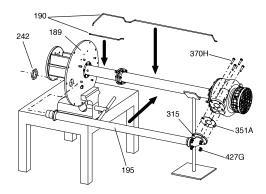
Figure 45: Discharge pipe reassembly
