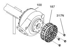
Figure 25: Strainer removal
