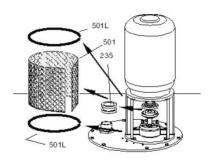
Figure 22: Coupling Guard Removal
