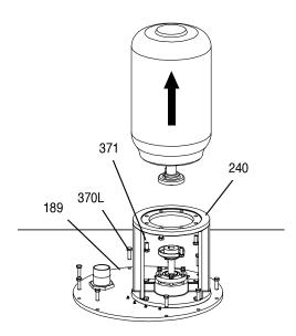
Figure 23: Motor Bolts Removal
