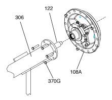
Figure 30: Adapter Removal
