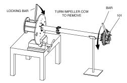
Figure 28: Impeller Removal
