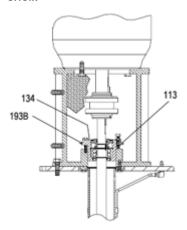
Figure 21: Thrust bearings
