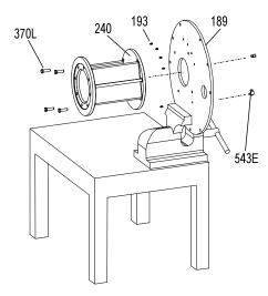
Figure 35: Motor Adapter Removal
