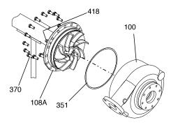
Figure 26: Casing Removal
