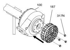
Figure 46: Strainer reassembly
