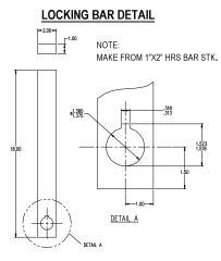
Figure 27: Locking Bar Detail
