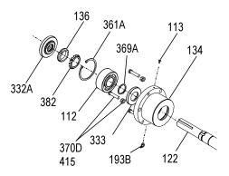
Figure 39: Retainer ring reassembly
