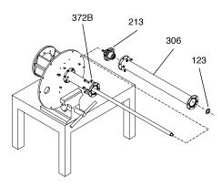
Figure 31: Column Removal
