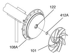
Figure 29: Impeller Removal
