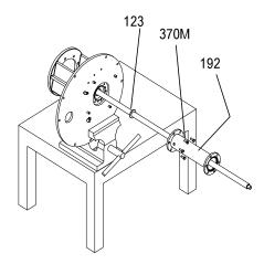
Figure 32: Head Column Removal
