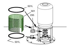
Figure 48: Coupling guard reassembly 15. Lubricate the pump bearings.
