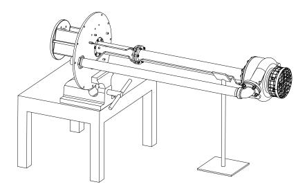
Figure 24: Lay Pump Horizontally on Proper Supports
