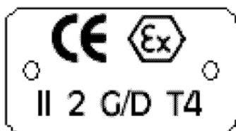
Figure 1: Typical ATEX pump nameplate
