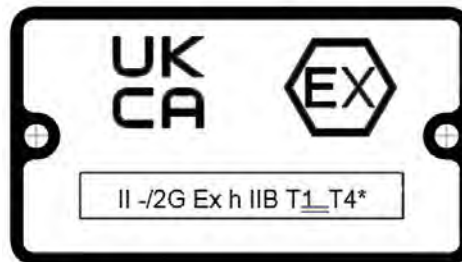
Figure 2: Typical UKCA ATEX nameplate
