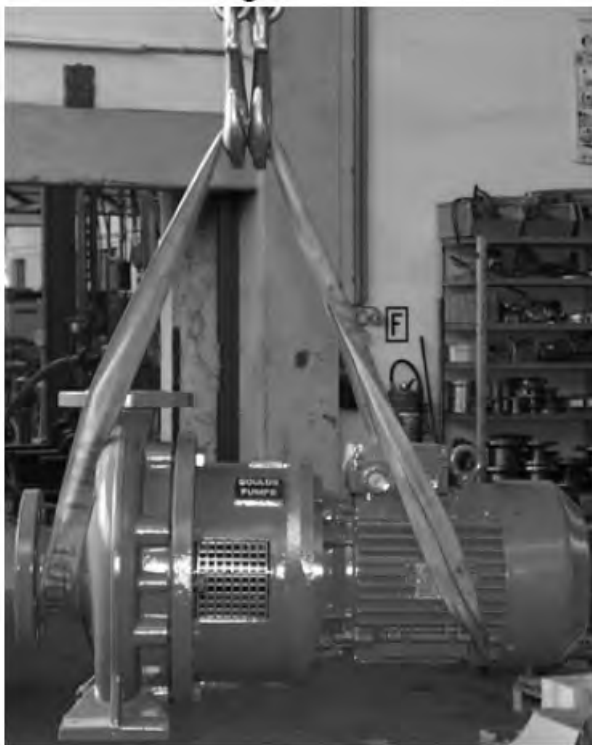
Figure 2: Levage de pompe
