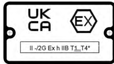
Figure 2: Typical UKCA ATEX nameplate
