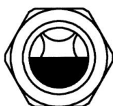
Figure 28: Oil level sight glass
