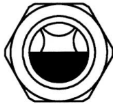
Figure 28: Oil level sight glass
