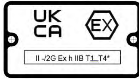
Figure 2: Typical UKCA ATEX nameplate
