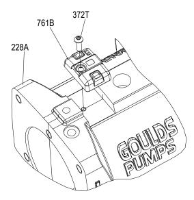
2. Tighten the hex-head screw with a 5/32 inch hex wrench to 6 ft-lbs (8 Nm).
