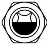
Figure 29: Oil level sight glass
