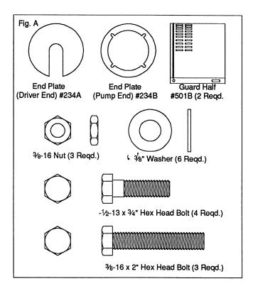
Simplicity of design allows complete assembly of the coupling guard, including the end plate (pump end), in about fifteen minutes. If the end plate is already in place, assembly can be accomplished in about five minutes.
