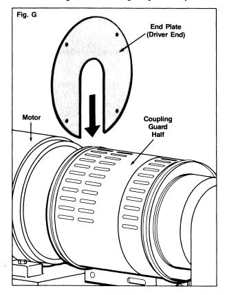
6. Adjust length of coupling guard to completely cover shafts and coupling as shown in Figure H by sliding coupling guard half (driver end) towards motor. After adjusting guard length, secure with bolt, nut and two (2) washers through the slotted holes at the center of the guard and tighten. Check all nuts on the guard assembly for tightness.
