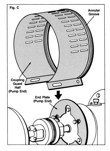
3. After the coupling guard half (pump end) is located around the end plate, secure it with a bolt, nut and two (2) washers through the round hole at the front end of the guard half as shown in Figure D. Tighten securely. See detail drawing, Figure E.
