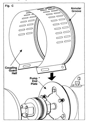
After the coupling guard half (pump end) is located around the end plate, secure it with a bolt, nut and two (2) washers through the round hole at the front end of the guard half as shown in Figure D. Tighten securely. See detail drawing, Figure E.
