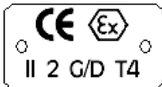
Figure 1: Typical ATEX pump nameplate
