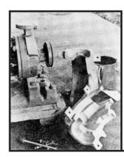
After pump is piped in line, assemble jacket, bolts, and standard heat transfer cement.
