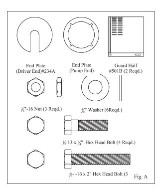
Simplicity of design allows complete assembly of the coupling guard in about five minutes.
