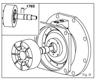
15. Carefully roll adapter with rotary assembly onto face of rotary assembly (impeller end of shaft facing up).
