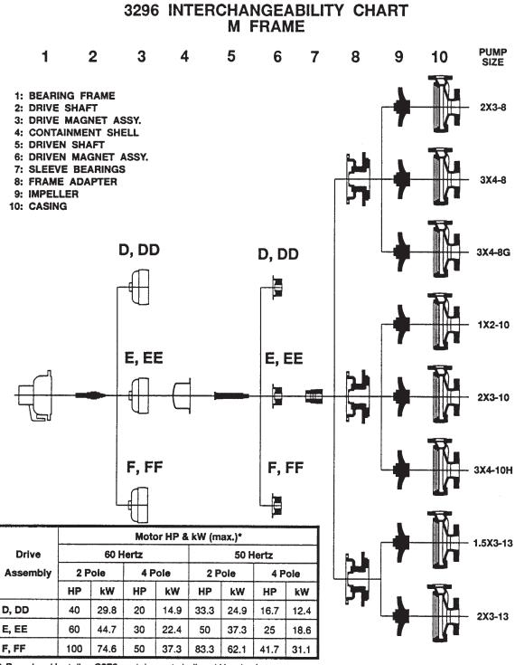
Based on Hastelloy C276 containment shell and Neodymium Iron (Drives D, E, F) or Samarium Cobalt (Drives DD, EE, FF) magnets.
