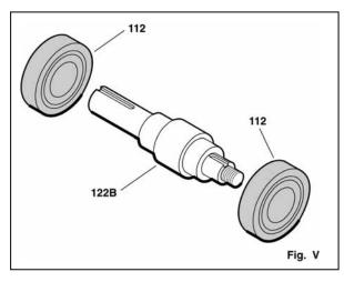
*NOTE:* There are several methods used to install bearings. The preferred method is to use an induction heater that heats as well as demagnetizes the bearings.
