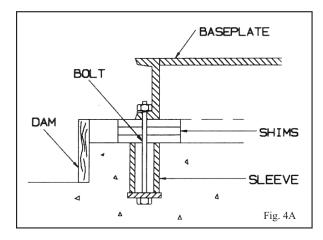
absorb any vibration and to form a permanent, rigid support for the pumping unit.
