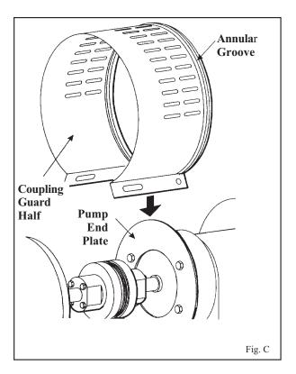
3. After the coupling guard half (pump end) is located around the end plate, secure it with a <sup>3</sup>/<sub>8</sub> - 16x2" hex head bolt, nut and two (2) washers through the round hole at the front end of the guard half as shown in Figure D. Tighten securely. See detail drawing, Figure E.
