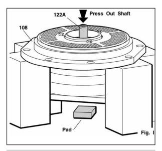
NOTE: Outboard rotary sleeve bearing will remain on shaft.
