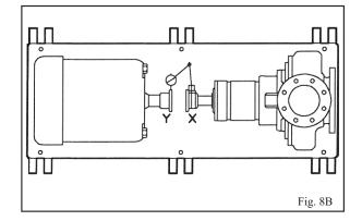
*NOTE:* Failure to slide motor evenly will affect horizontal angular correction.
