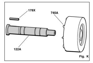
19. Wrap driven magnet assembly (740A) in a clean cloth to keep clean and set aside away from attracting metals.
