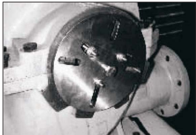
Figure 15: Removing bearing and gland plate using universal fixture
