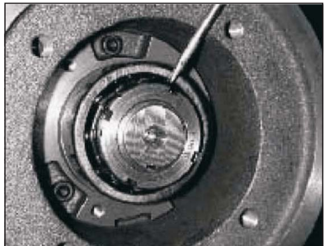
Figure 20: Installing Lockwasher and Locknut
