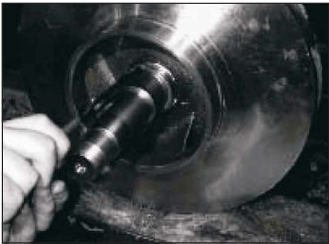
Figure 22: Removing Impeller Retaining Ring
