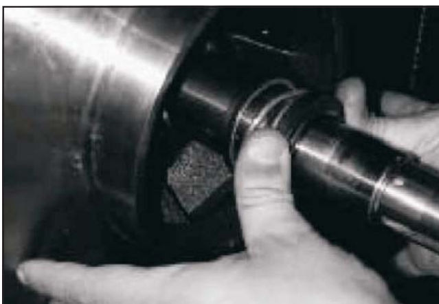
Figure 25: Installing Mechanical Seal Head
