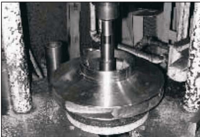
Figure 24: Pressing Impeller on Shaft
