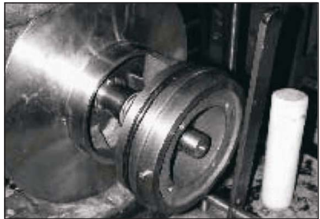
Figure 26: Installing Stuffing Box
