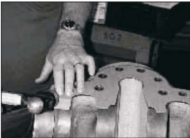
Figure 23: Trimming Casing Gasket
