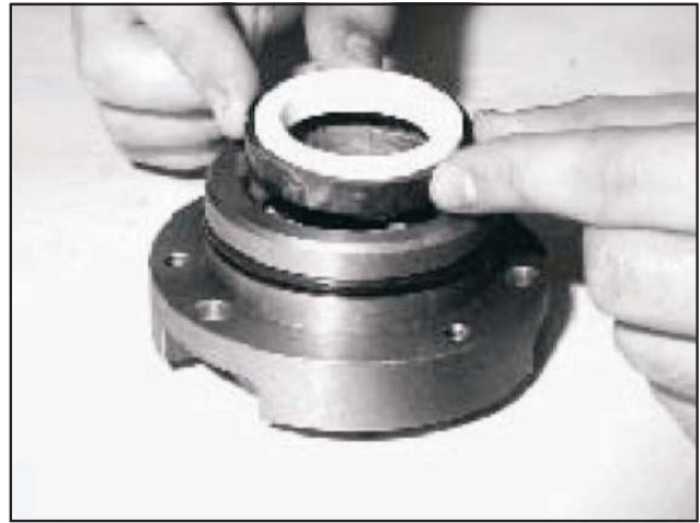
Figure 17: Assembling mechanical seal seat into gland plate
