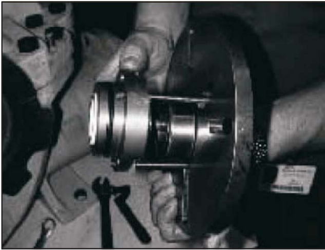
Figure 16: Gland plate and bearing removed from stuffing box
