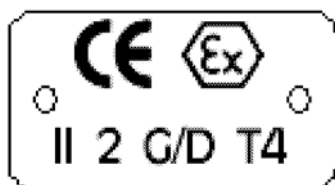
Figure 1: Typical ATEX pump nameplate
