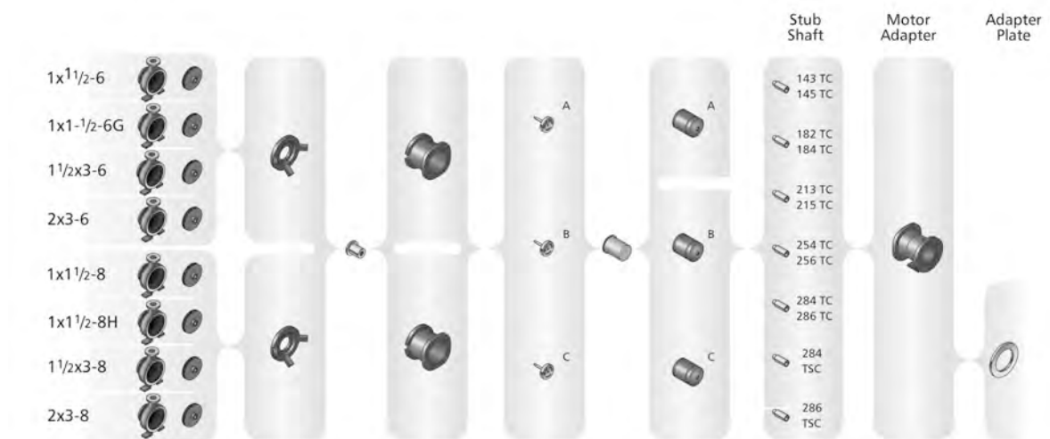
Figure 36: Accouplement direct 3296 EZMAG
