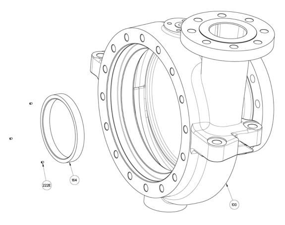
Figure 62: Casing wear ring
