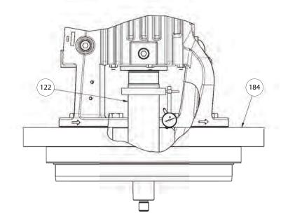
Figure 78: Seal-chamber lock (register) runout
