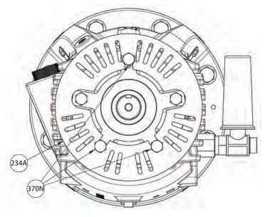
Figure 23: Thrust bearing end cover removal
