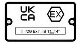
Figure 11: Typical UKCA Ex nameplate
