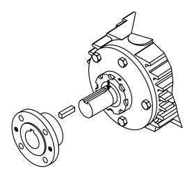
Figure 80: Coupling hub installation
