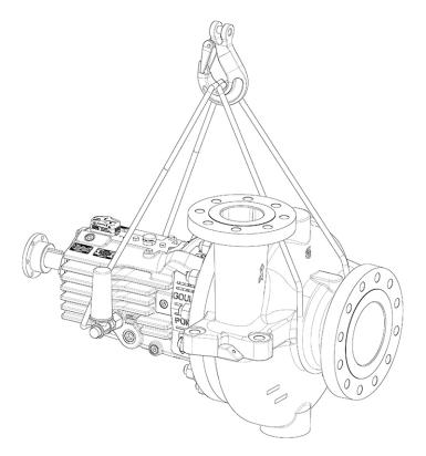
Figure 3: Example of a proper lifting method of pump with driver
