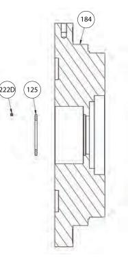
Figure 63: Seal chamber cover wear ring and throat bushing
