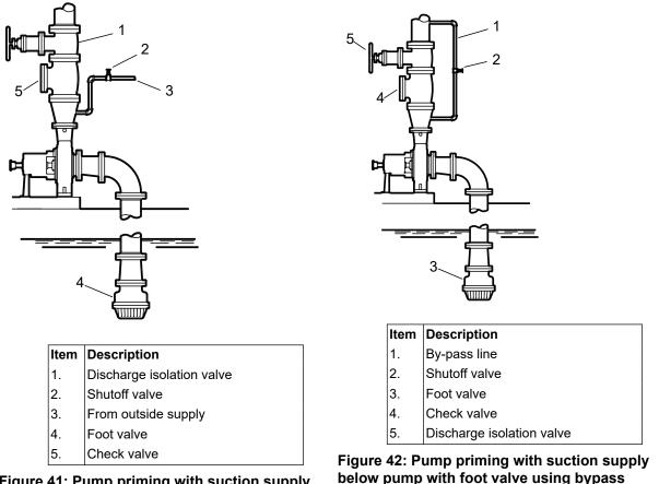
Figure 41: Pump priming with suction supply below pump with fo below pump with foot valve and an outside sup- around check valve ply
