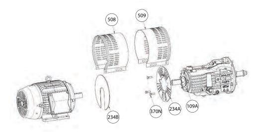
Figure 21: Coupling guard removal
