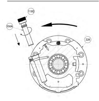
Figure 36: New filter installation
