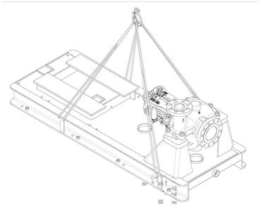
Figure 4: Example of a proper lifting method of pump and driver on base plate
