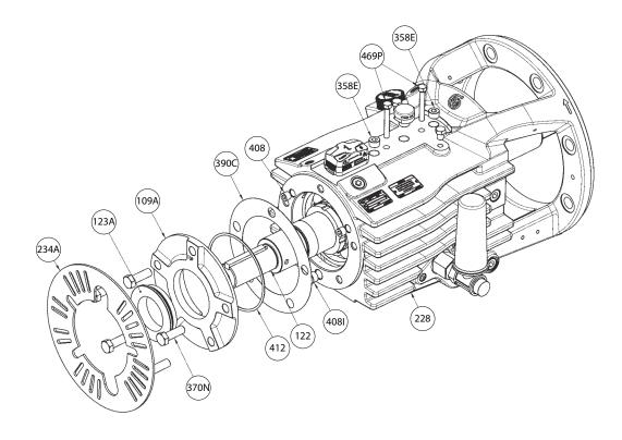
Figure 50: Thrust cover removal
