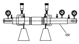
Figure 57: Shaft inspection
