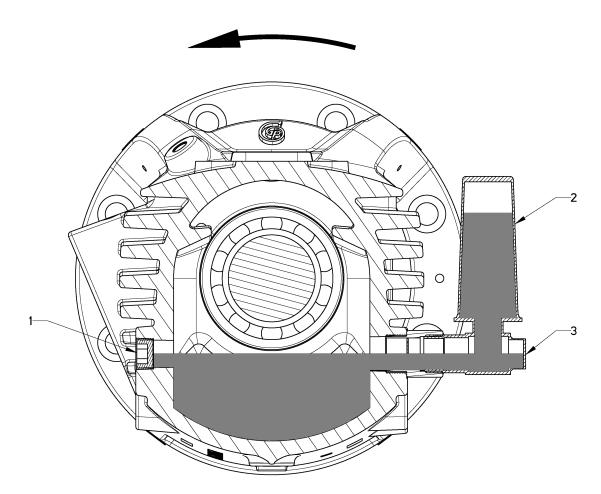
Figure 32: Checking oil level
