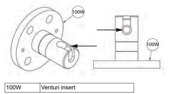
Figure 56: Venturi insert inspection
