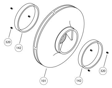
Figure 61: Replace impeller wear ring
