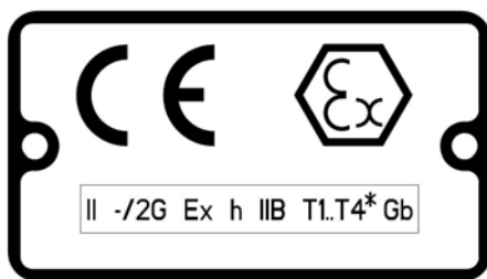
Figure 1: Plaque signalétique Ex typique
