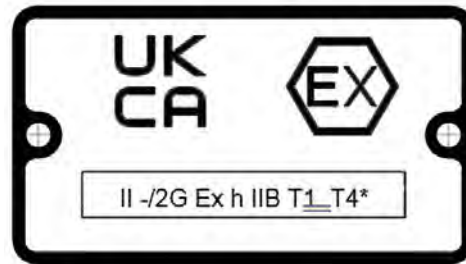
Figure 2: Typical UKCA Ex nameplate
