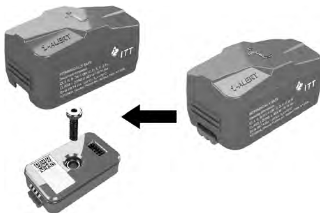
Figure 25: Disengage the battery from the sensor when shutting the pump for an extended period of time
