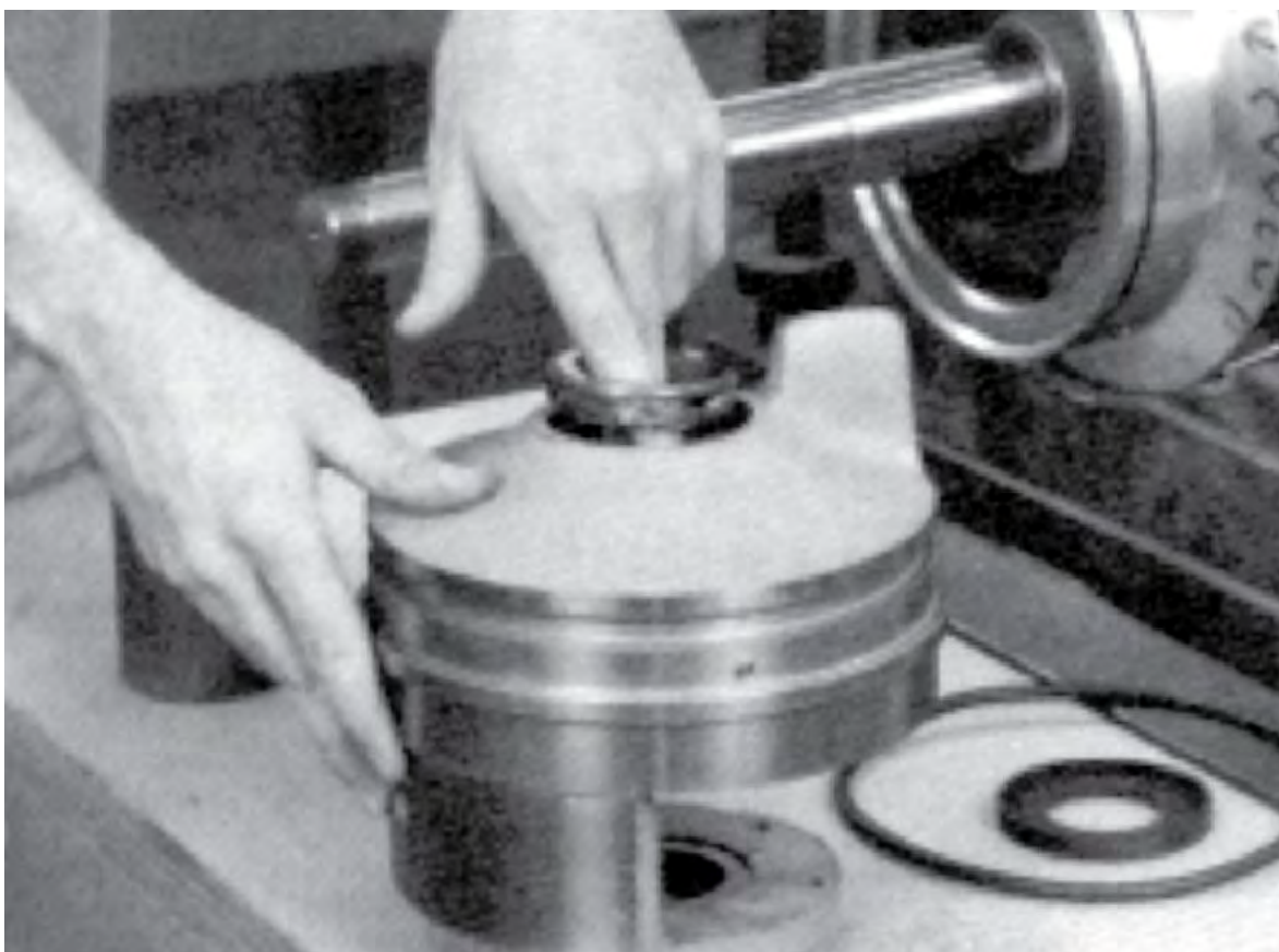
Figure 49: Press mechanical seal stationary seats into stuffing boxes
