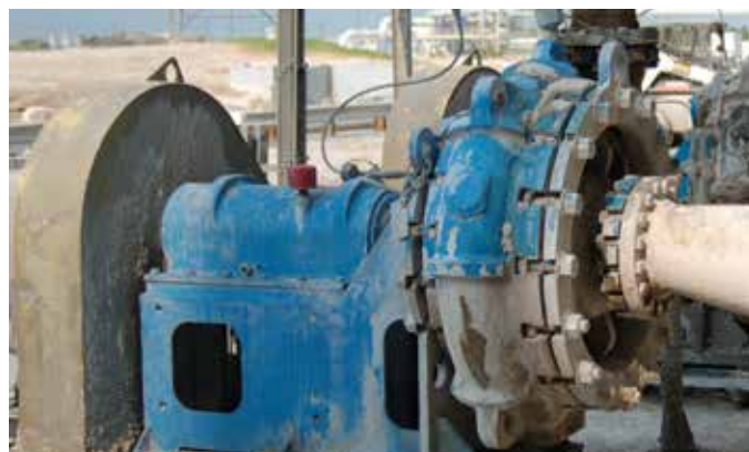
Model 5500 pumping Phosphogypsum in a phosphate plant.
