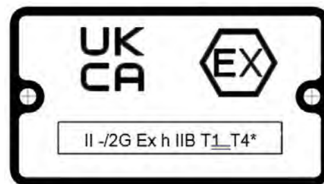
Figure 8: Typical UKCA Ex nameplate
