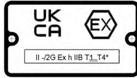
Figure 2: Typical UKCA Ex nameplate
