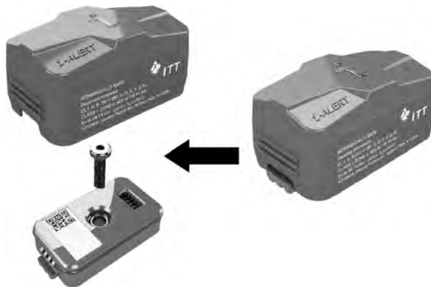
Figure 24: Disengage the battery from the sensor when shutting the pump for an extended period of time
