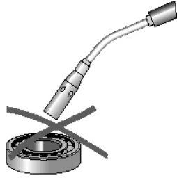
Figure 48: Do not use torch to heat bearings
