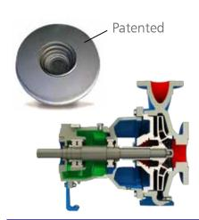
The number one cause of pump downtime is failure of the shaft seal. Typically, seal failures are the result of an unfavorable seal environment such as poor heat dissipation, poor lubrication or operation in the presence of solids or vapors.
