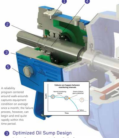
Internal sump geometry is optimized for longer bearing life. Sump size increased by 10%-20% results in better heat transfer and cooler bearings. Contoured design directs contaminants away from bearings, to the magnetic drain plug for safe removal.
