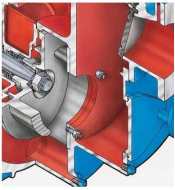
The large capacity priming chamber retains plenty of liquid for consistent priming and repriming.
