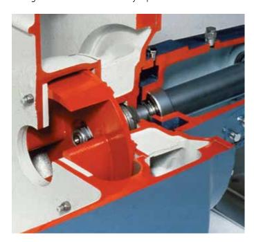
The power end is supported by a rigid cast iron frame foot that provides excellent support for the shaft and thrust bearing. Bearing life is extended.
