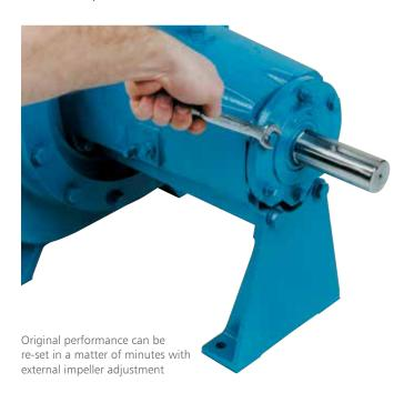
Adjustable cartridge style bearing housing allows adjustment of impeller to wearplate clearance. No shims are required. No need to disassemble or drain pump.
