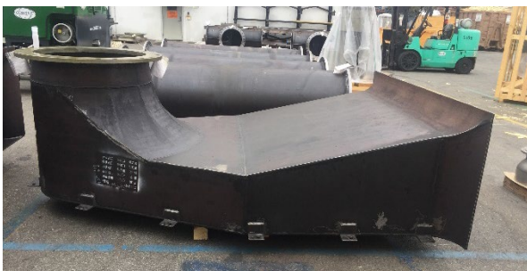
Finished Fabricated Form Suction Intake
