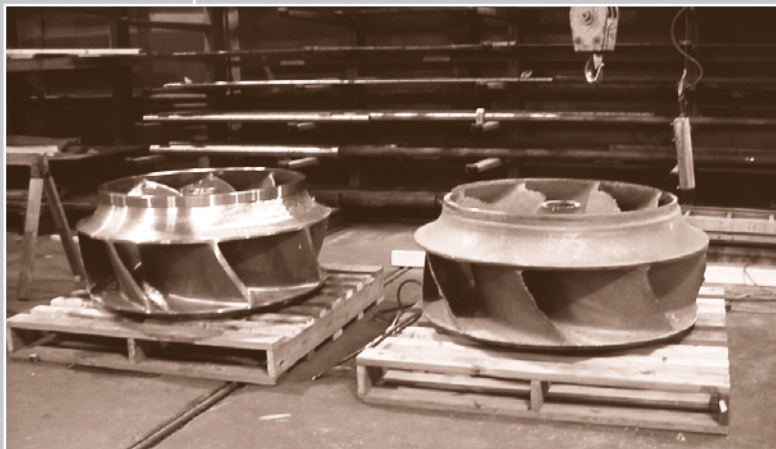
(3) week turnaround on this 60" Foster Wheeler Circ Water Vertical. Right is the old bronze impeller. Left is the new 316SS impeller.
