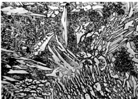
Typical CD-4M Cu alloy. Solution annealed at 2000°F.
