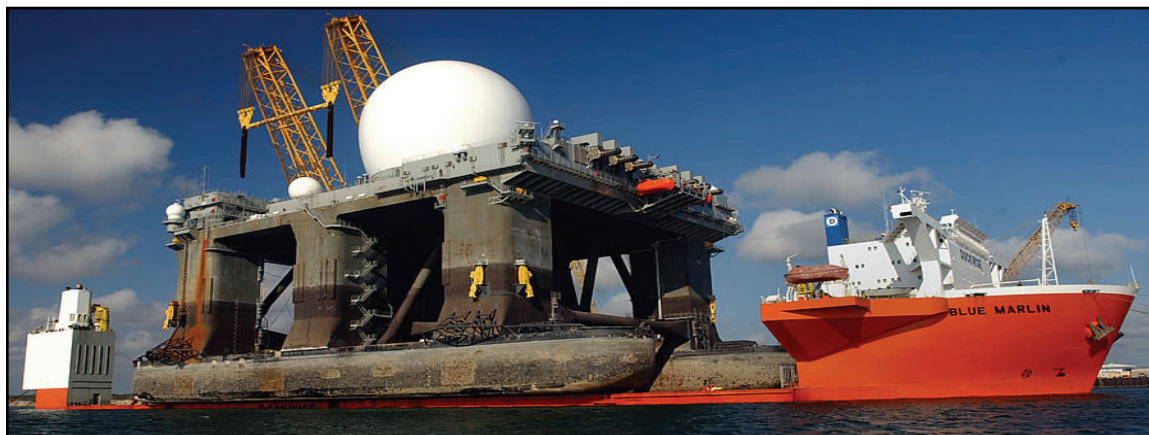
The Sea-Based X-Band Radar (SBX) on the heavy lift vessel MV Blue Marlin
