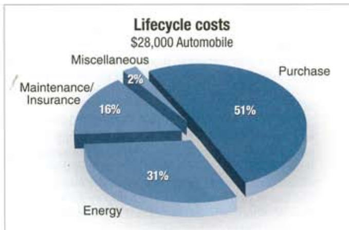
Fig. 1. Fuel is nearly one-third of a car's life cycle cost, whereas the purchase price accounts for more than half.
