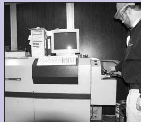
Figure 2. Metallurgical Laboratory ARC/Spark Optical Emission Spectrometer (OES). Used to determine chemical composition and create certified material test reports.
