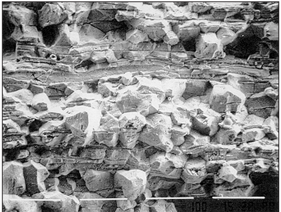
Fractograph illustrates Hydrogen-Induced fracture in a UNS S41600 martensitic stainless steel component. Magnification 200X.
