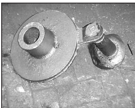
Figure 5, The casting ready for cleaning
