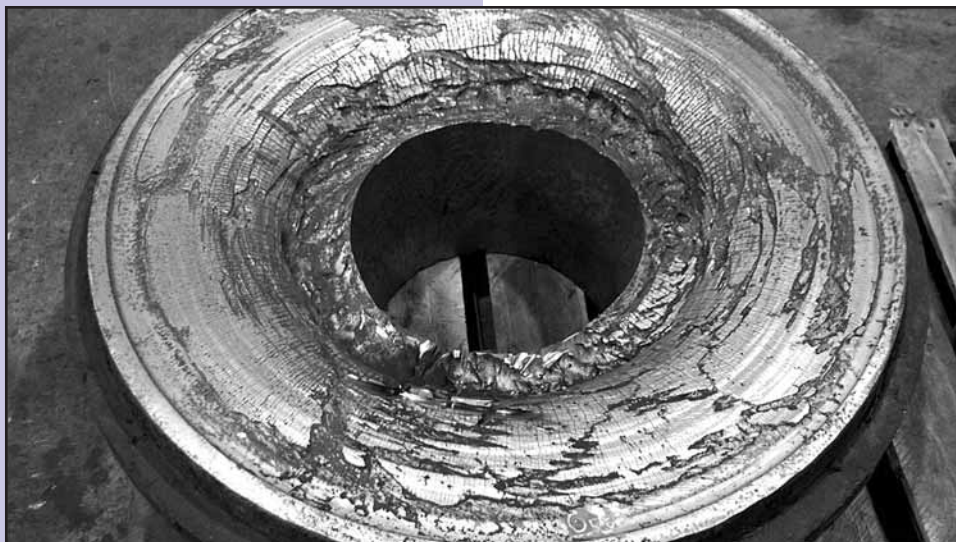
Figure 1. Condition of the severely damaged suction cover
