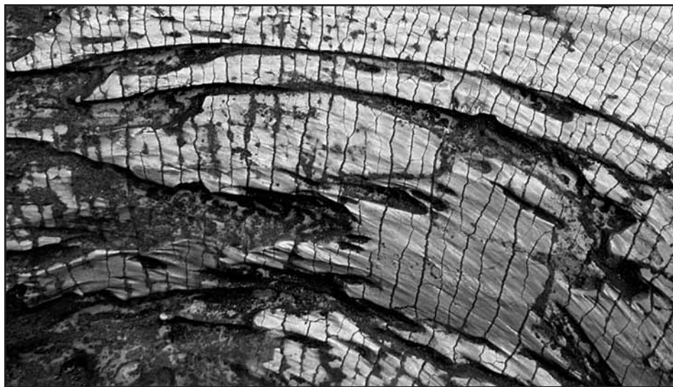
Figure 2. Close-up of extensive "Heat checking" characteristic of thermal fatigue cracking.
