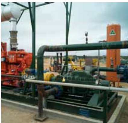
Model 3600 (BB3) in a water injection service located in a demanding western Australian Desert.
