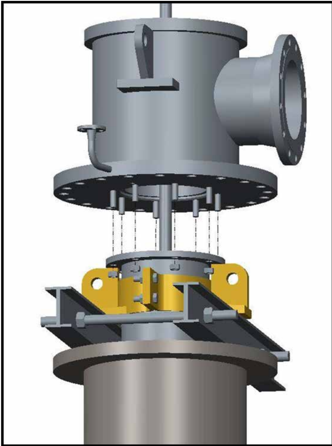
Figure 22: Discharge Head lowering.
