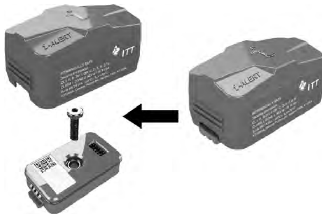
Figure 41: Disengage the battery from the sensor when shutting the pump for an extended period of time
