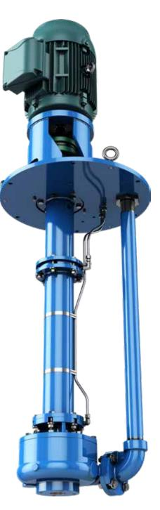
The CV 3171 is a recessed impeller, circular volute type sump pump. Ideal for large solids and shear sensitive fluids. It will pass any solid that will pass through the discharge pipe. Circular volute minimizes radial loads, making this the ideal pump for low flow process applications.
