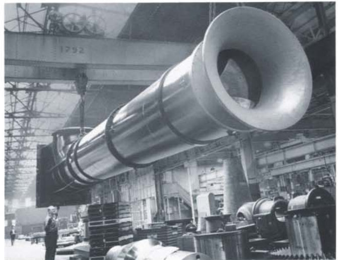
Vertical Wet-Pit Column Pump being prepared for shipment.
