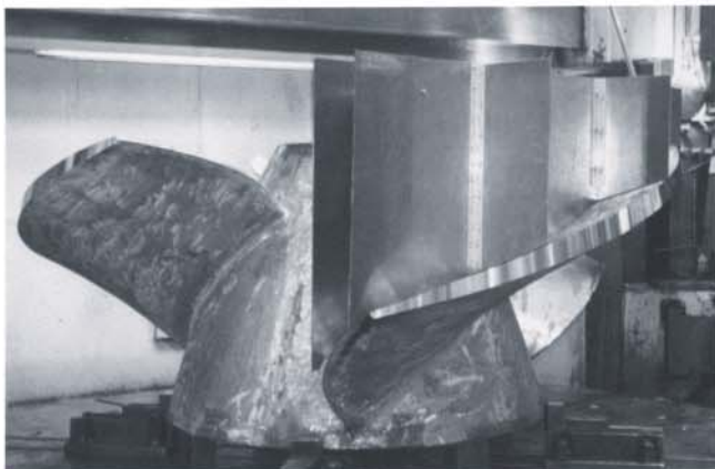
A semi-open impeller being checked with a vane template to assure geometrical similarity to the manufacturing drawing.
