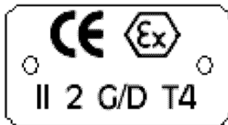
Figure 1: Typical Ex pump nameplate
