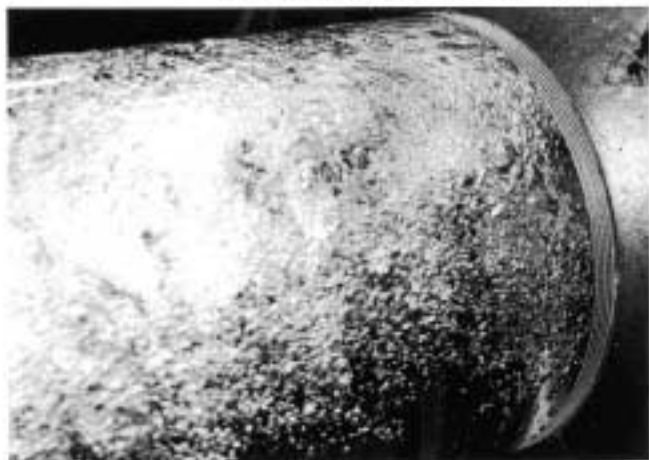
Figure 9. Transparent Suction Pipe with Six Percent Entrained Air by Volume, at Best Efficiency Point, 1780 RPM.
