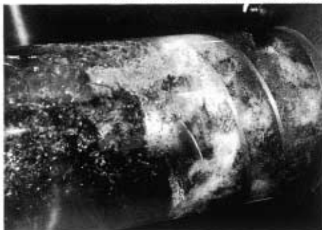
Figure 16. Inducer with Six Percent Entrained Air at 50 Percent of Best Efficiency Point, 1180 RPM.
