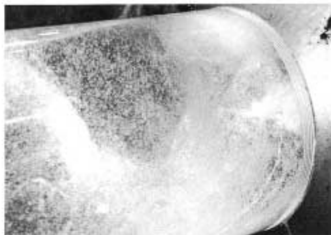
Figure 10. Transparent Suction Pipe with Six Percent Entrained Air by Volume, at 20 Percent of Best Efficiency Point, 1780 RPM.
