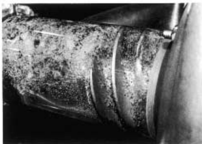
Figure 15. Inducer with Six Percent Entrained Air at 75 Percent of Best Efficiency Point, 1180 RPM.
