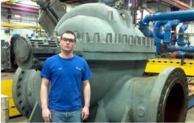
Brazil Refinery - Crude Transfer Pipeline 30x36-32 600 psi (42 Bar), 3500 HP (2600 kW)
